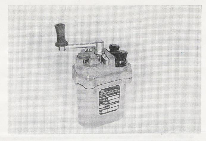
The exploder ECA300A is an extremly reliable crank charged condenser blasting machine developed for using under rough conditions. It is suited for firing series of about 300 A - bridge detonators (4 mJ/ohm) with 3,5 m copper wires respectively 100 U - bridge detonators (16 mJ/ohm).
